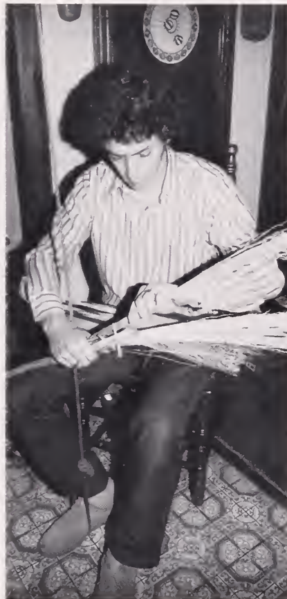
Wooden pegs through the end of maple handle anchor the twine and help hold the sweeps. Notice how the sweeps are being fitted between the pegs. (John McGinley pictured.)
